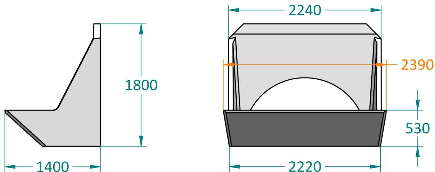
The dimension in red gives the distance from the PE 1000 bubbler sill level to the INVERT of the Maxiflow.
