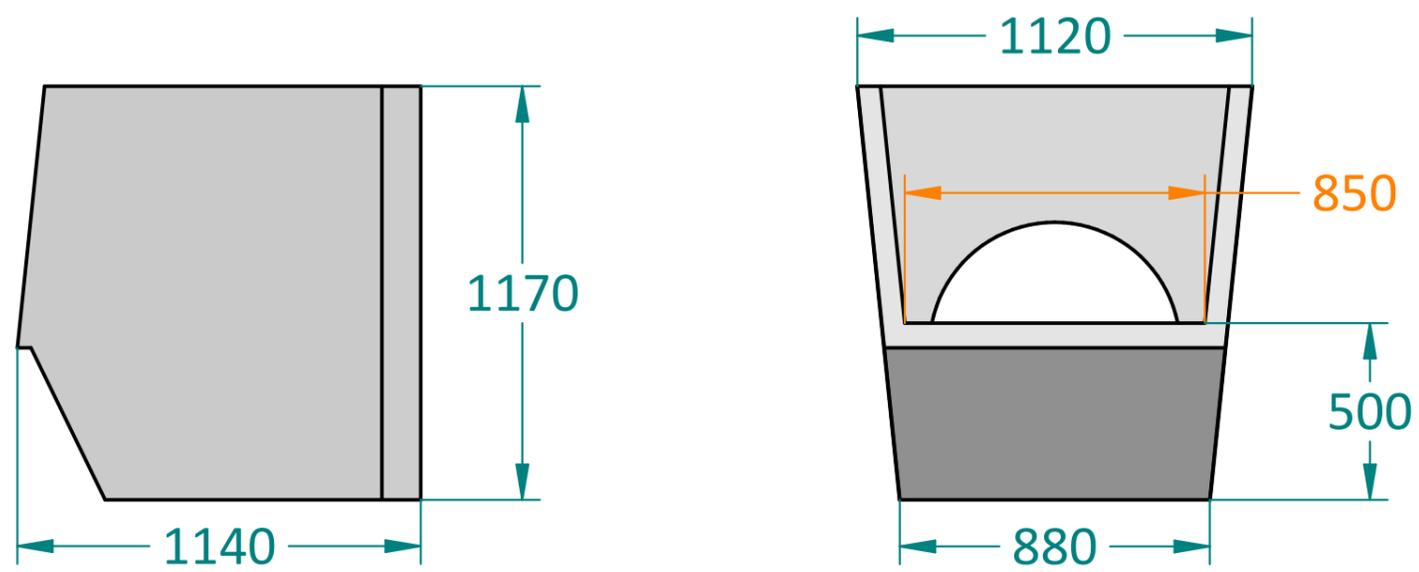
The dimensions in red give the distance from the PE 600 sill level to the INVERT of the pipe.
