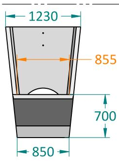
The dimensions in red give the distance from the PE 600-1000 sill level to the INVERT of the pipe.
