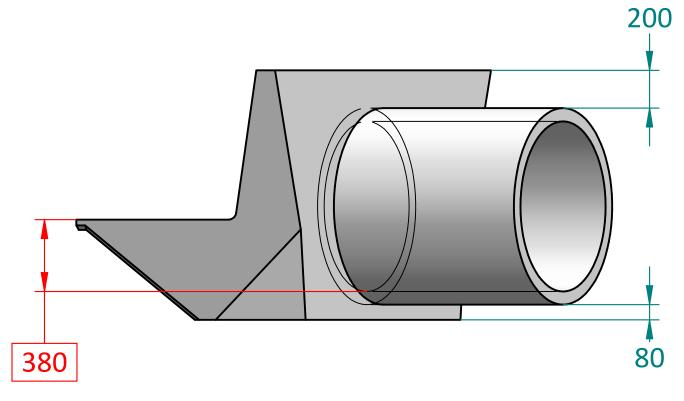
The dimension in red gives the distance from the PE 900 bubbler sill level to the INVERT of the pipe.
