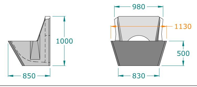
The dimension in red gives the distance from the PE 450 bubbler sill level to the INVERT of the pipe.
