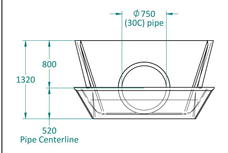
The dimension in green gives the distance from the top of the PE 900 bubbler to the top of the pipe.
