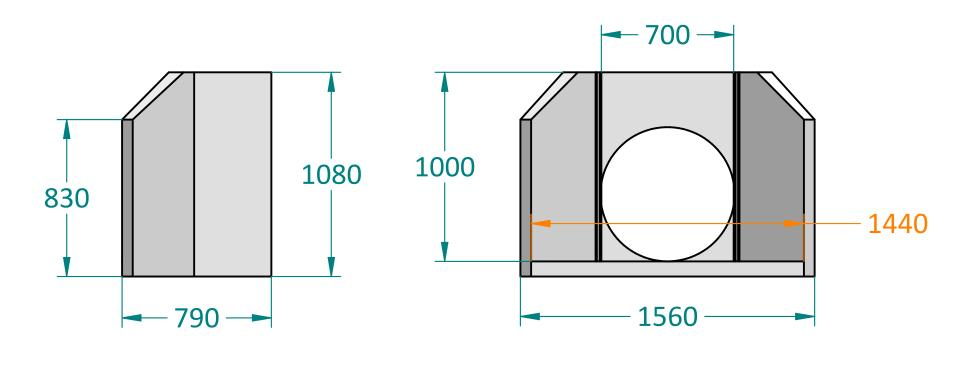
The dimension in red gives the distance from the top of the RH 1000 to the INVERT of the pipe.
