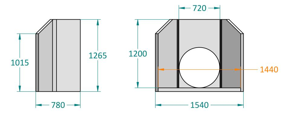
The dimension in red gives the distance from the top of the RH 1200 to the INVERT of the pipe.
