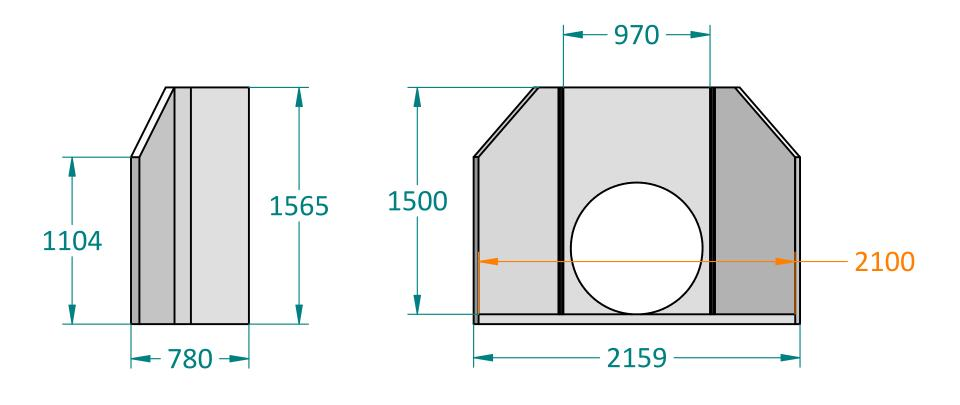
The dimension in red gives the distance from the top of the RH 1500 to the INVERT of the pipe.
