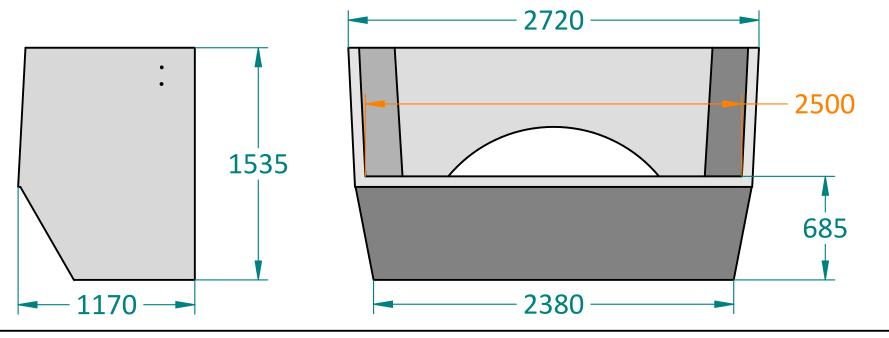
The dimension in red gives the distance from the PE 1000 sill level to the INVERT of the Maxiflow.
