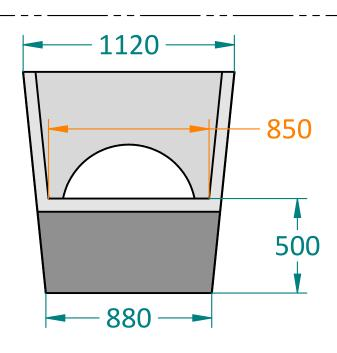
The dimensions in red give the distance from the PE 600 sill level to the INVERT of the pipe.
