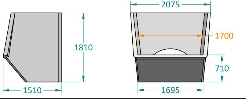
The dimension in red gives the distance from the PE 900-1000 sill level to the INVERT of the Maxiflow.
