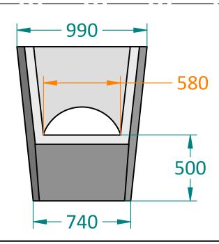
The dimensions in red give the distance from the PEXL sill level to the INVERT of the pipe.
